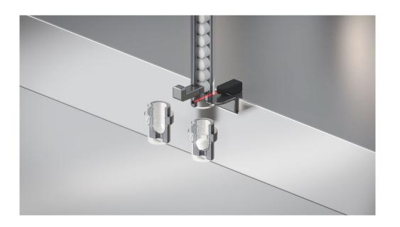
The unit can introduce one or more **tablets/soft gel/hard gelatin capsules** into the capsule body in one stroke, using a blade and feeding tubes.
