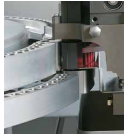
Sensor to check tablet/capsule presence
